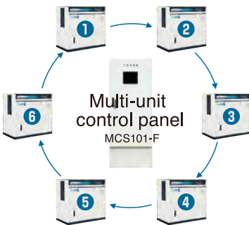
Schematic diagram of rotary operation
